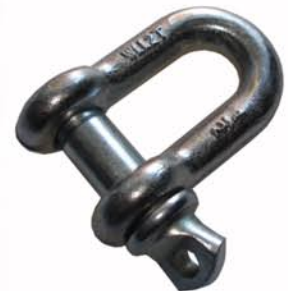
JS-DSH08R D Shackle 8mm rated 0.75T JS-DSH10R D Shackle 10mm rated 1.00T JS-DSH11R D Shackle 11mm rated 1.5T JS-DSH13R D Shackle 13mm rated 2.0T JS-DSH16R D Shackle 16mm rated 3.25T JS-DSH19R D Shackle 19mm rated 4.75T
