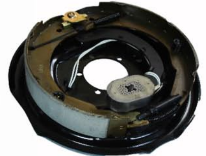
JS-EBKH12 Backing Plate 12" Electric
