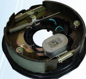
JS-EBKH10 Backing Plate 10" Electric
