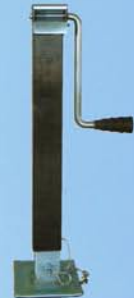
JS-SJAK7-E Square Jack Cap: 7000Lbs Extendable Height: 615mm Travel 15"+13.6"
